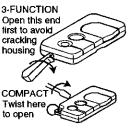
control case.) Insert batteries positive side down.
